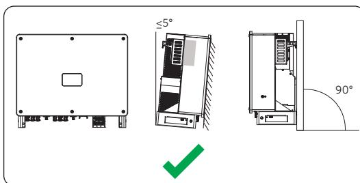
Figure 6-1 Correct installation
