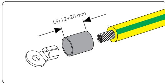
Figure 7-4 Installing the tubing and OT terminal
