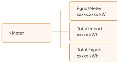
The user can check the active power received from the meter and import/export energy by this function. There are three parameters: **Pgrid/Meter**, **Total Import** and **Total Export**. Press **Up** and **Down** to review the values. If no meter is connected, the parameters here will display 0.
