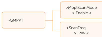
This interface is used to configure GMPPT settings, including MPPT scan mode and scan frequency.
