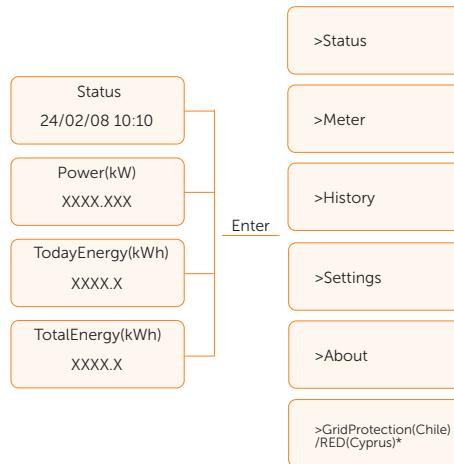
The main interface (Level 1) is the default interface, the inverter will automatically jump to this interface when the system started up successfully or not operated for a period of time.
