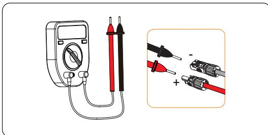
Figure 7-57 Measuring the voltage of PV connectors
