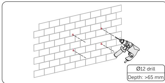
Figure 6-13 Drilling holes
