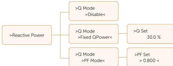
This interface is used to set the reactive power. Please set the value according to the requirement of utility grid.
