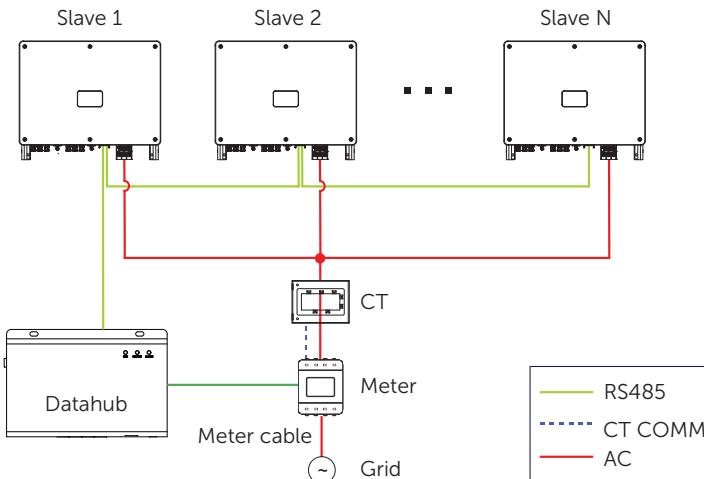
Figure 14-2 Parallel system diagram with Datahub
