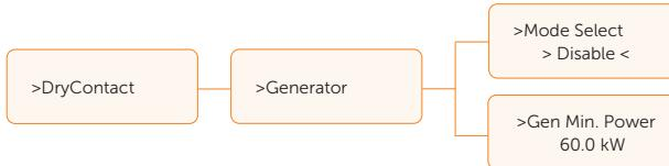
The user can select the operational mode and set the generator's minimum power output. You can also press **Mode Select** to choose to disable the generator.
