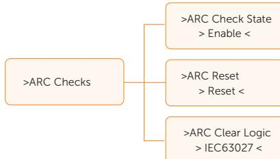
If the ARC reset is enabled after an arc fault occurs, the fault will be automatically removed after a short period of time and the machine will resume; if it is not, the fault will always be there and must be fully disconnected from the power source in order to recover.
