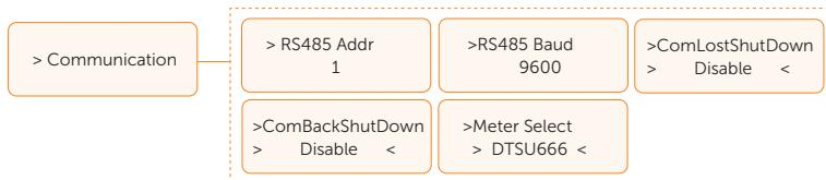
**RS45 Addr** and **RS45 Baud** are the primary communication settings for RS45 which can be configured to 1 and 9600.
