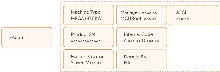
This interface shows information of the inverter, include model, SN, software version of master DSP, slaver and ARM board and internal code.
