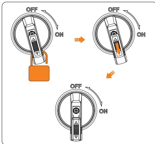
Figure 8-8 Unlocking the DC switch
