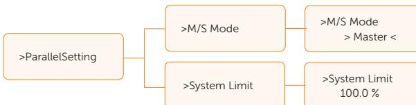
**M/S Mode** can choose **Master** or **Slave**. **System Limit** can set whether to allow the reverse flow power from inverter to power grid, and the default value is 0%. Check [14.2 Application of Parallel Function](#) for detailed settings.
