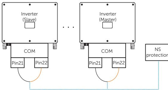
Figure 9-4 Connection diagram for NS Protection in parallel
