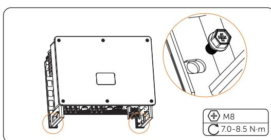
Figure 6-11 Securing the inverter
