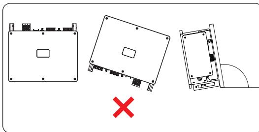
Figure 6-2 Incorrect installation
