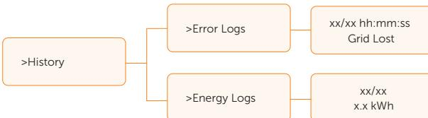
The user can check the error logs and energy logs by this function.
