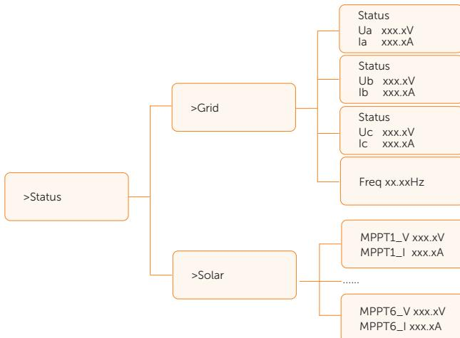
The status function contains **Grid** and **Solar**. Press **Up** and **Down** to select and press **Enter** to confirm the selection. Press **ESC** to return to menu.
