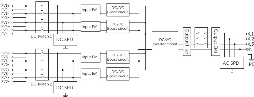
Figure 2-5 Circuit diagram for inverters of 25 kW / 40 kW
