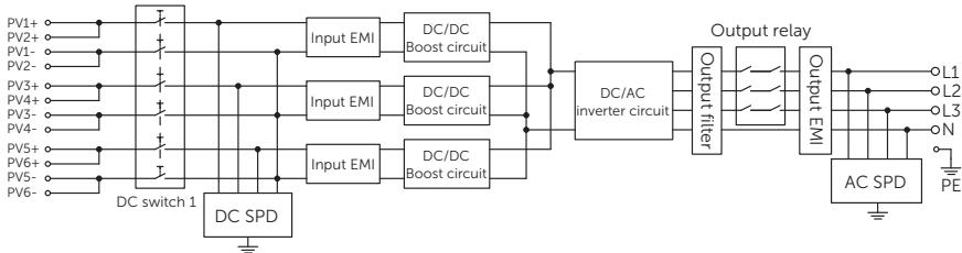
Figure 2-4 Circuit diagram for inverters of 20 kW
