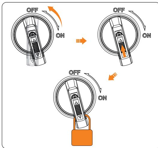
Figure 8-7 Locking the DC switch
