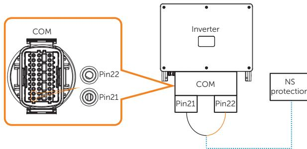
Figure 9-3 Connection diagram for NS Protection
