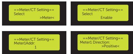
Figure 14-9 Setting meter for the inverter
