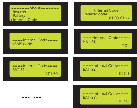
Figure 9-105 Displaying the internal code information
