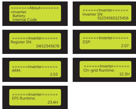
Figure 9-103 Displaying the inverter information
