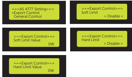
Figure 9-70 Setting export control in AS4777 setting interface
