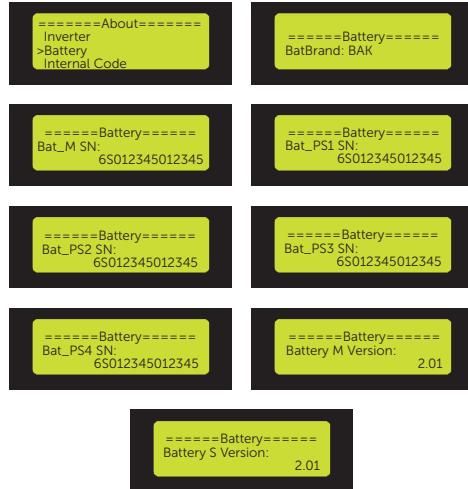
Figure 9-104 Displaying the battery information
