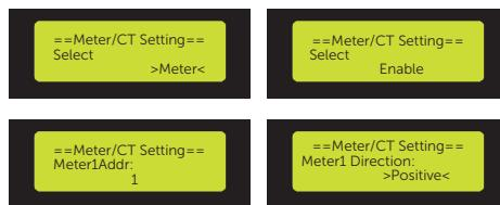
Figure 14-14 Setting meter for the inverter
