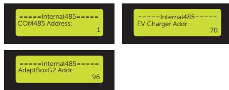
Figure 9-94 Setting the address of the external device
