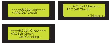
Figure 9-101 Triggering ARC Self Check
