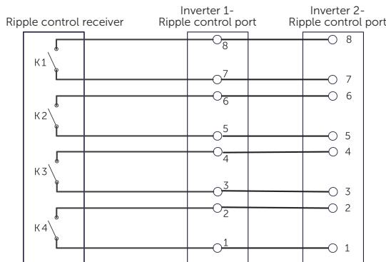
Figure 8-59 Connection diagram for ripple control in parallel
