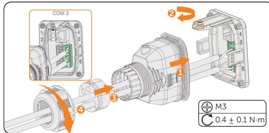
Figure 8-65 Connecting to the inverter
