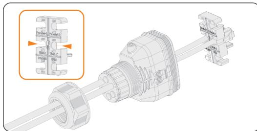
Figure 8-42 Installing RJ45 terminal to the cable fixture
