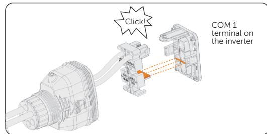
Figure 8-39 Inserting the connector to COM 1
