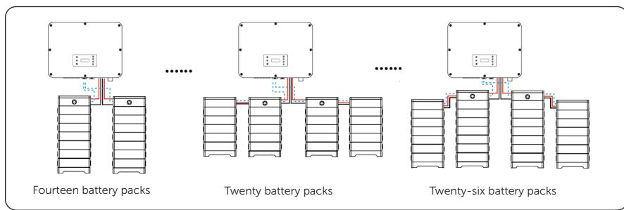
Figure 8-25 Battery connection Scheme 2
