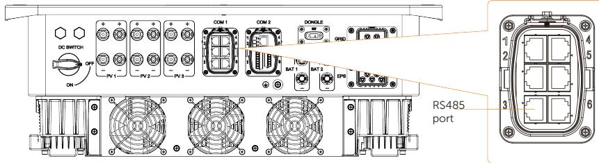
Figure 15-11 Connection port for DataHub
