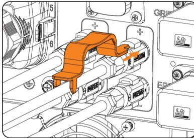
Figure 13-4 Removing the Battery connector
