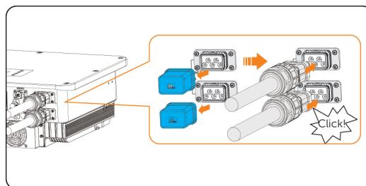
Figure 8-13 Installing the AC connector to inverter
