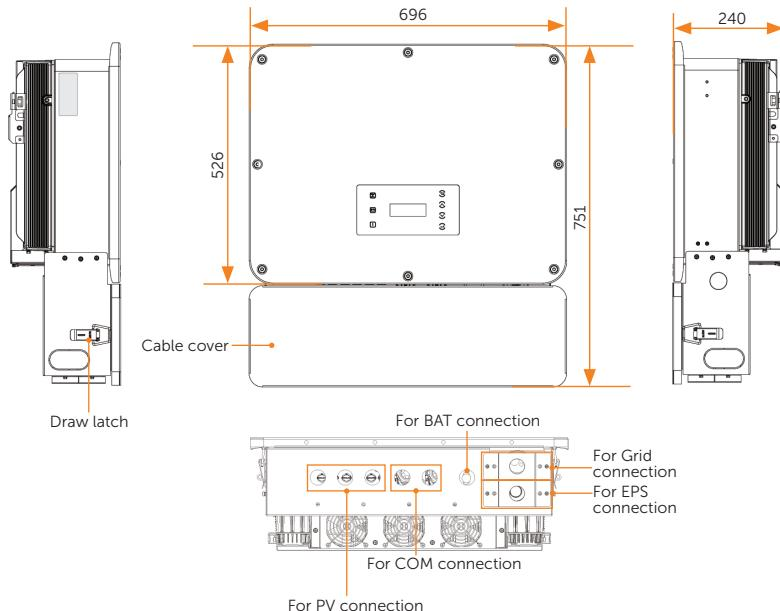
Figure 15-23 Appearance with cable cover (Unit: mm)
