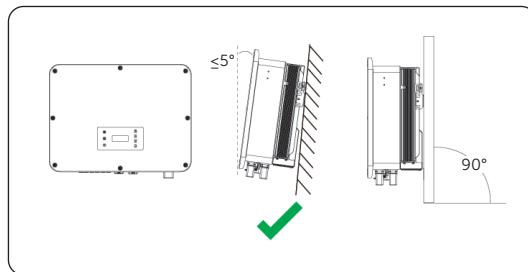
Figure 7-1 Correct installation
