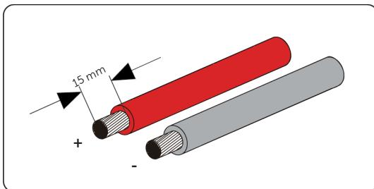
Figure 8-29 Striping the battery cable
