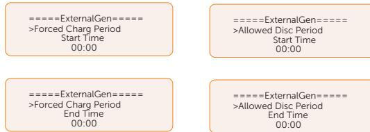
» **Allow Work:** Allowed time period for generator operating. You can set the start time and end time.
