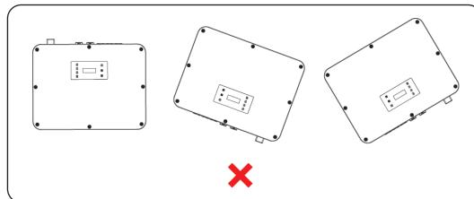
Figure 7-2 Incorrect installation
