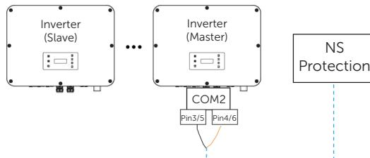
Figure 10-10 Connection diagram for NS Protection in parallel
