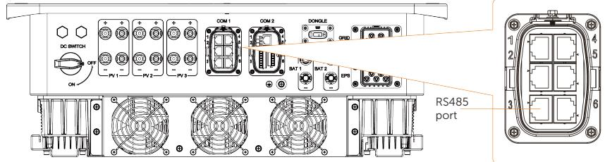
Figure 15-5 Connection port for Adapter Box G2
