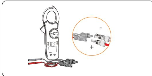
Figure 8-20 Measuring the voltage of PV connectors
