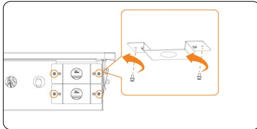
Figure 15-28 Loosening the screws from cable cover
